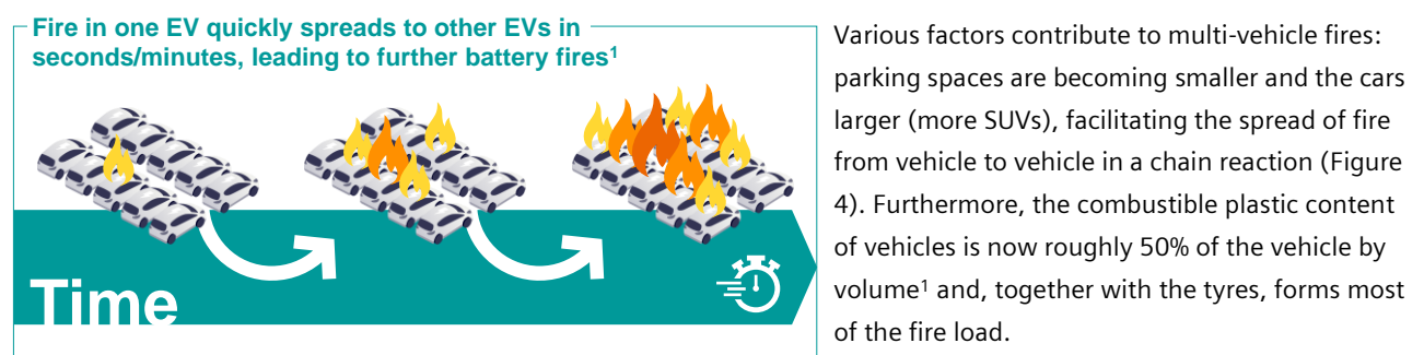
Figure 4: Fire quickly spreading from vehicle to vehicle
