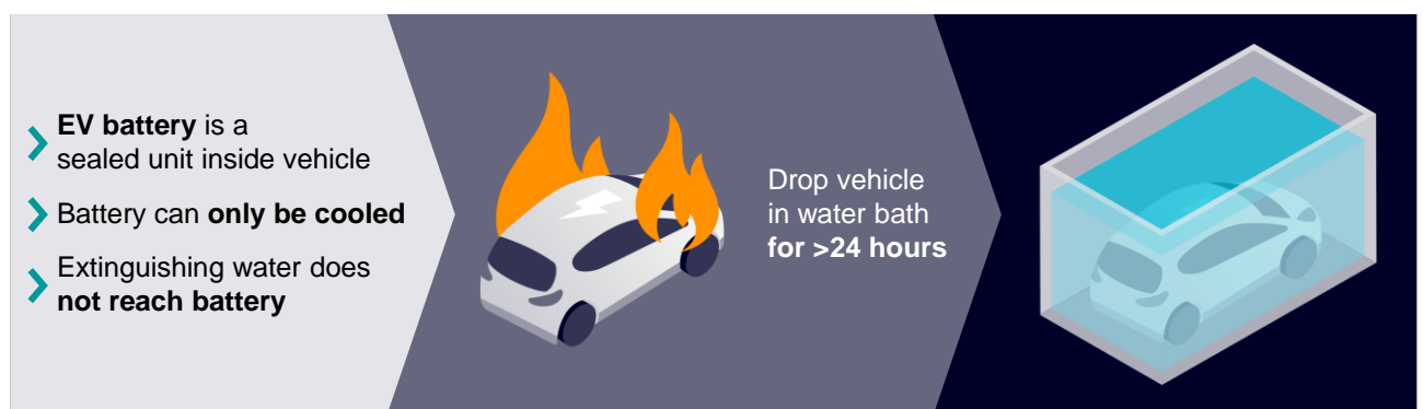
Figure 5: Water cooling of vehicles with battery fires
